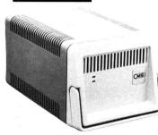
The CMS S-40 external hard-disk drive is one of the fastest Apple drives on the market and features an embedded SCSI controller.
